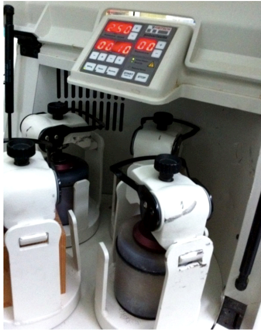
Figure 3.3 Ball milling for piezoelectric paint fabrication
