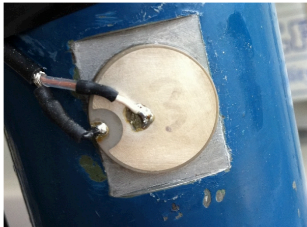
Figure 2.7 A piezoelectric ceramic sensor adhered on a steel tube
