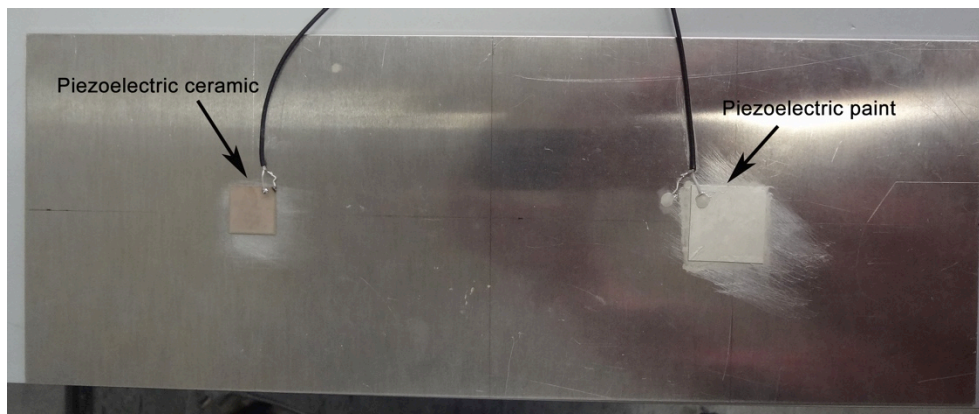
Figure 3.37 Piezoelectric ceramic and paint on an aluminum plate
