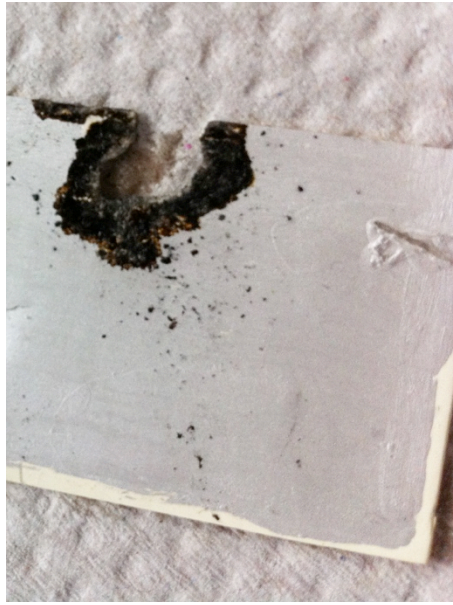
Figure 3.9 Dielectric break down during polarization
