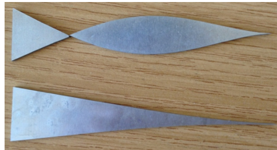
Figure 4.7 Aluminum molds used for modal sensor shaping
