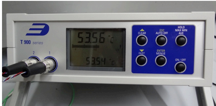
Figure 3.38 Series T900 process-controlled temperature measurement instrument
