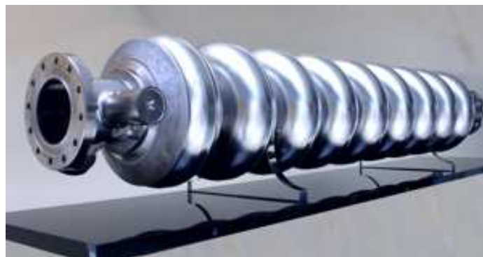
Figure 2.1: A TESLA-type cavity, fabricated from niobium, operating frequency 1.3 GHz (Courtesy FG-ISRF, HZB).
