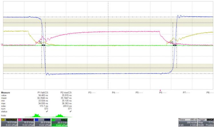
Abb. C.8: HEXFET:  $t_{\text{fall}}$ : s. P1 |  $t_{\text{rise}}$ : s. P2 |  $t_{\text{off}} = 147 \text{ ns}$  |  $t_{\text{on}} = 80 \text{ ns}$
