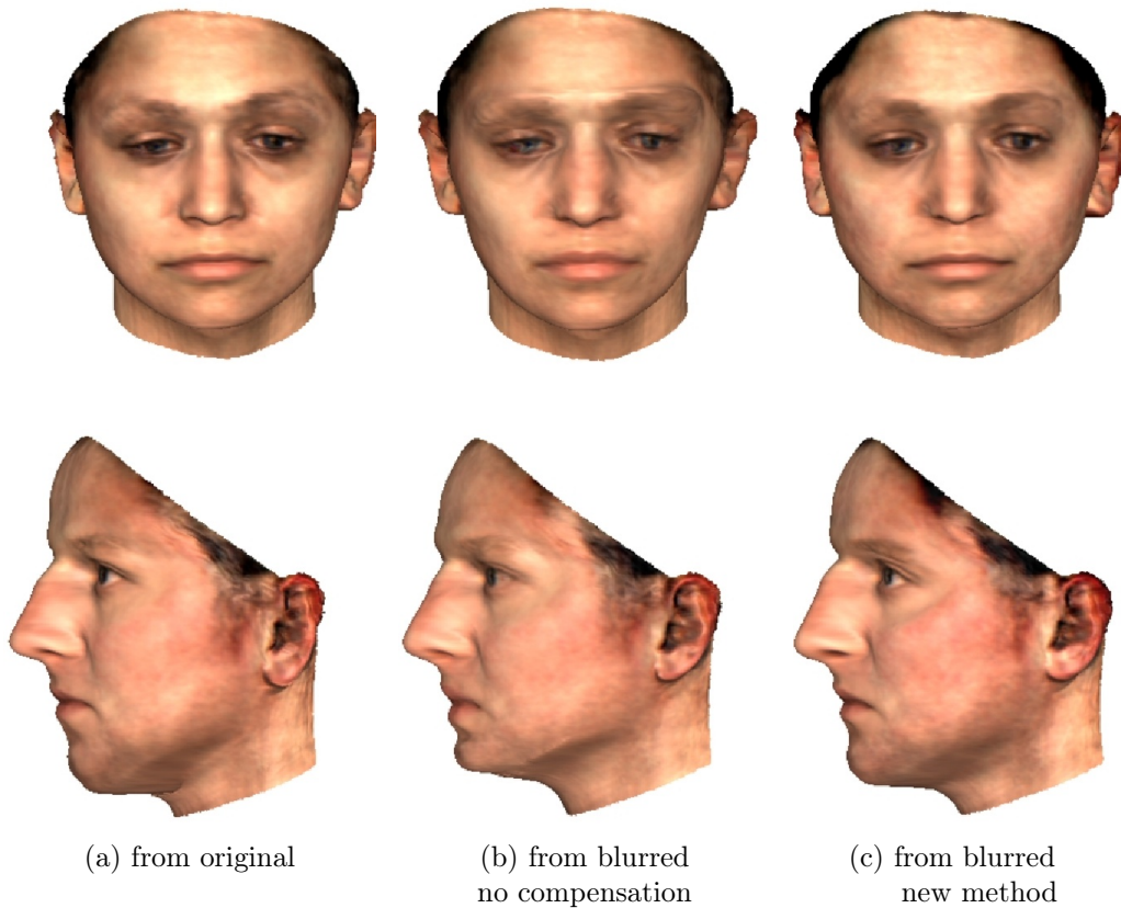
Figure 4.8: Comparison of blurred and unblurred reconstruction for shape: 3D face reconstruction from original unblurred image (left), blurred image without compensation (middle) and blurred image with the new method (right).
