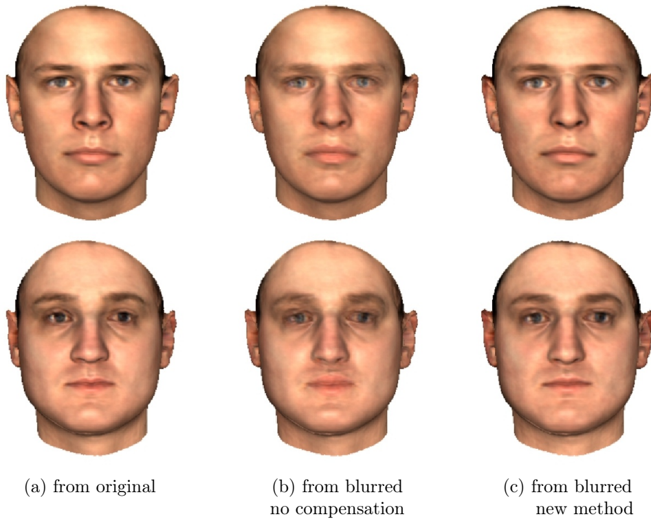
Figure 4.9: Comparison of blurred and unblurred 3D reconstruction for texture: 3D face reconstruction from original unblurred image (left), blurred image without compensation (middle) and blurred image with the new method (right).
