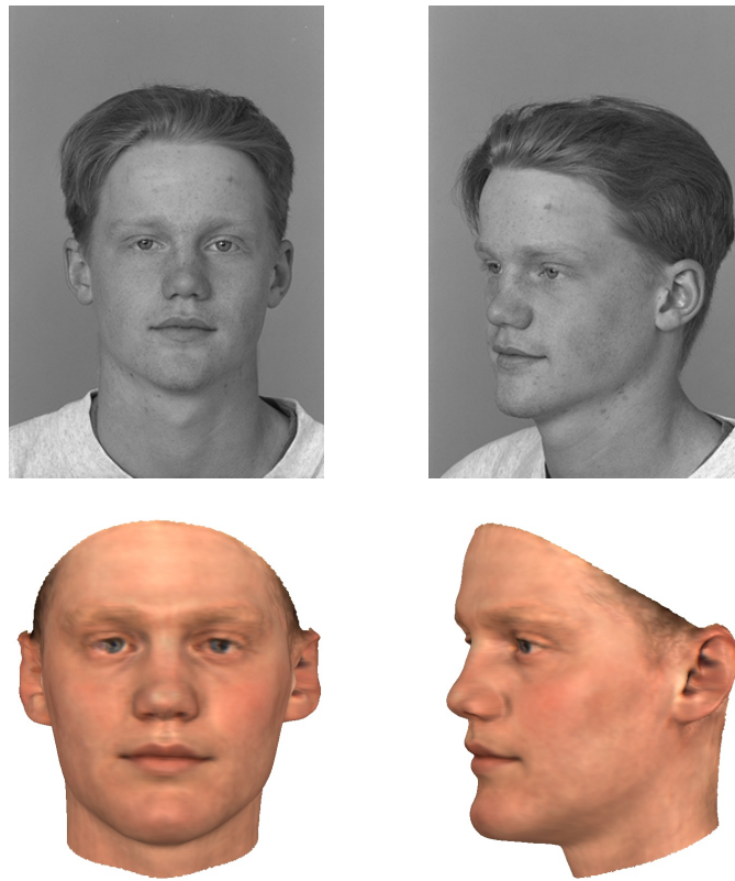
Figure 7.2: Multi-view reconstruction: The first row shows two portraits of the same person from different perspectives (taken from [PWHR98]). The bottom row depicts the 3D face reconstruction in two views where both frontal and side view images are used by the reconstruction algorithm simultaneously.
