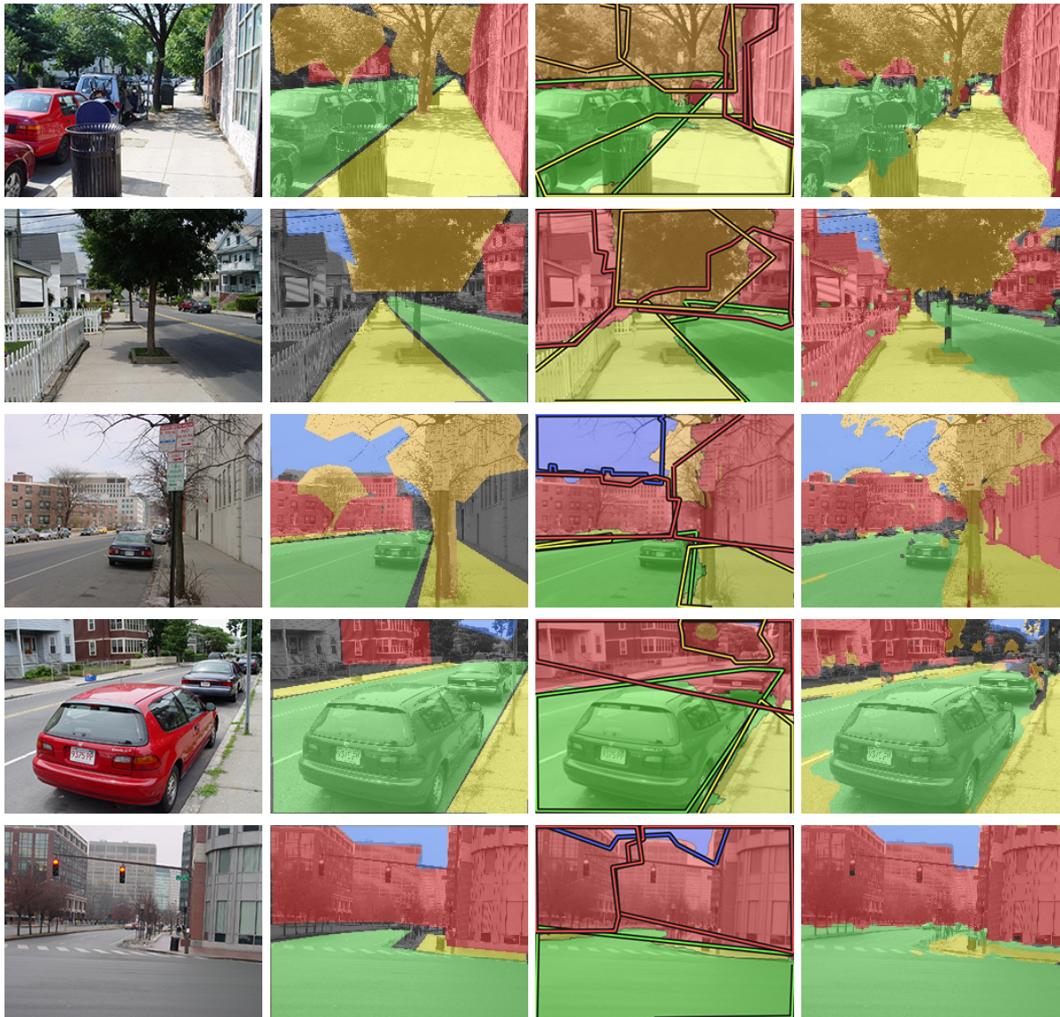
Fig. 3.17: Classification results on StreetScenes dataset: Left to right: Original image; Reference for base layer; Guo & Hoiem method with polygon fitting; ML-CRF. Green: road ; yellow: sidewalk ; red: building ; orange: tree ; blue: sky ; gray: unknown .
