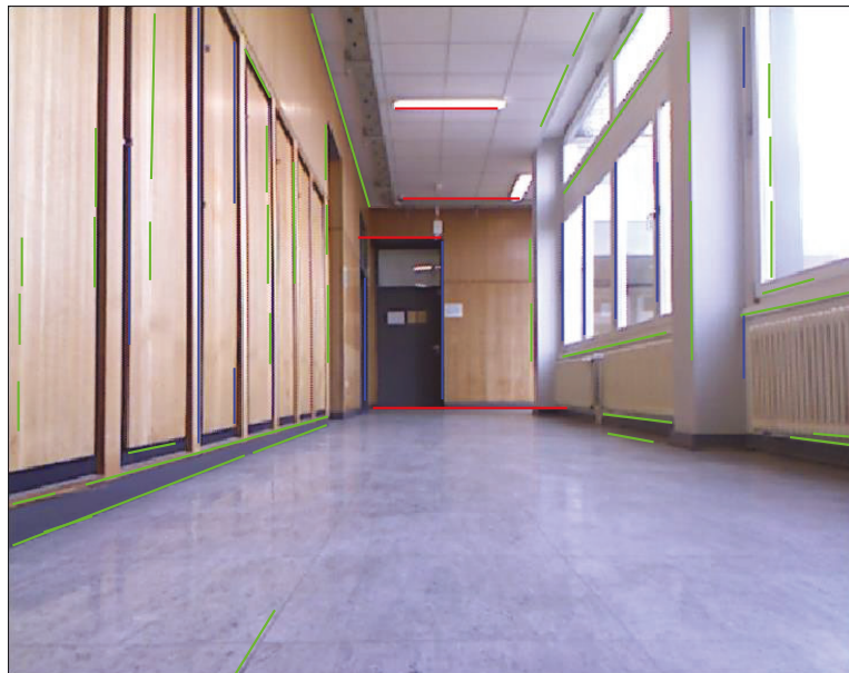
Figure 5.6: The results of line detection in the indoor environment
