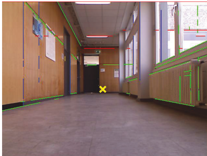
Figure 5.8: Localization of central vanishing point
