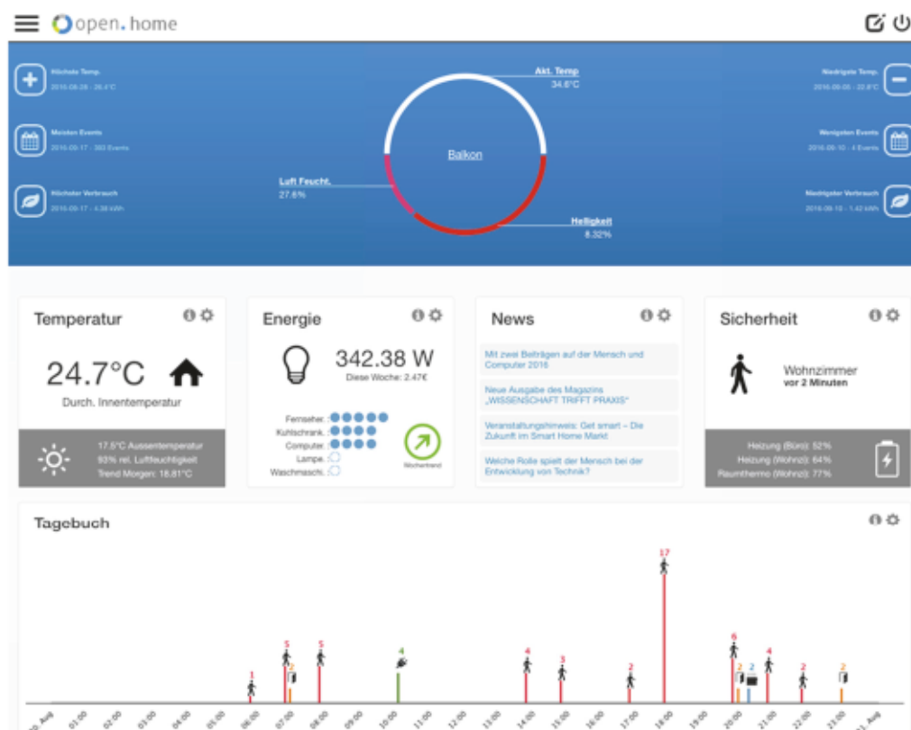
Figure 2: The home screen of the open.HOME interface with the first version of the system-awareness log at the bottom.
