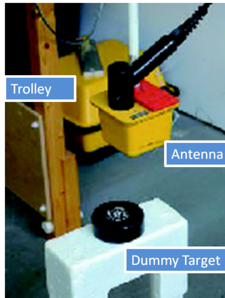
Figure 4.1 – The L-band GPR system is attached to a movable trolley platform. It is mounted along a rail system and scans the target from above.
