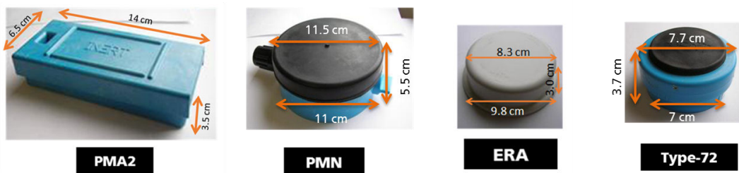
Figure 4.3 – Details of the simulant landmines and the standard test target buried in the test field.
