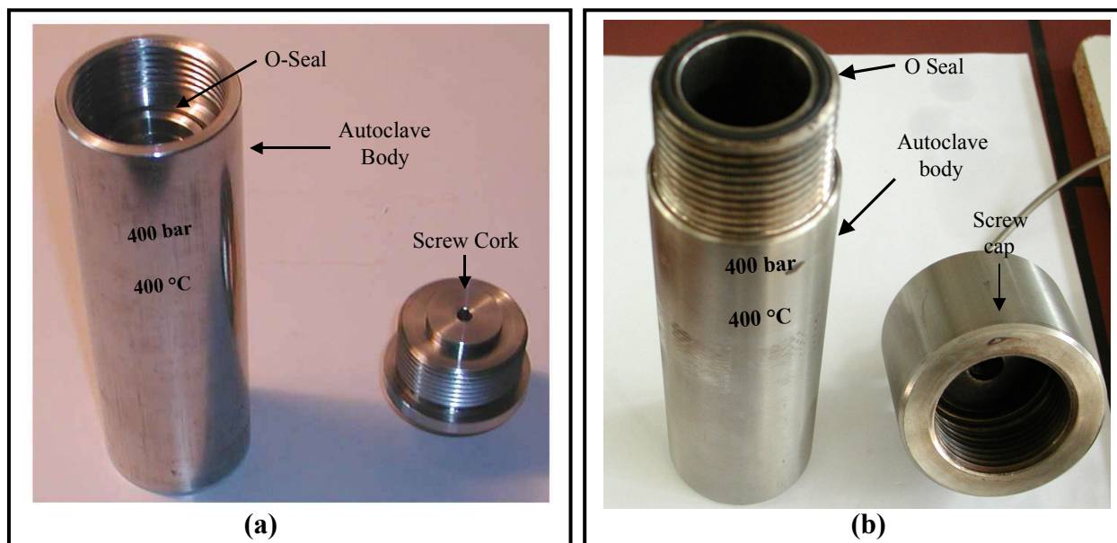
Fig. 3.10: Steel autoclaves used for the scCO_2 reactions.
