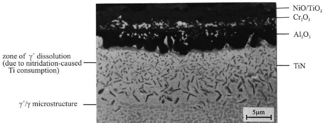
Figure 5.18: Cross-sectional micrograph of SC Ni-base superalloy SRR99 (approximately Ni-10W-8Cr-6Al-5Co-3Ta-2Ti in wt.%) after exposure to air at 1000°C for 100 h [107]
