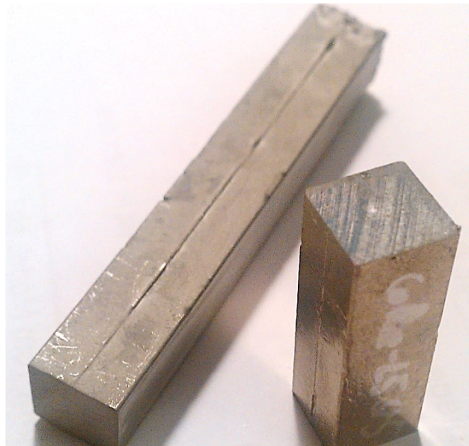
Figure 3.1: Cast alloy bar after heat treatments
