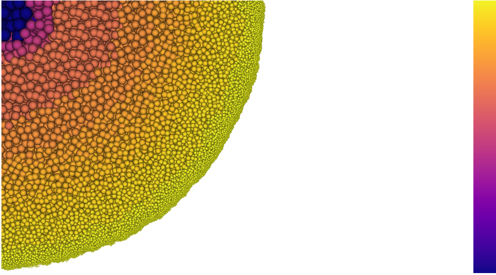
Figure 3.2: This image shows a cross section of the sphere in the sphere drop scenario where we used an adaptivity ratio of 1:10000. Mass is color coded from purple m^{\text{base}} to yellow m^{\text{fine}} .
