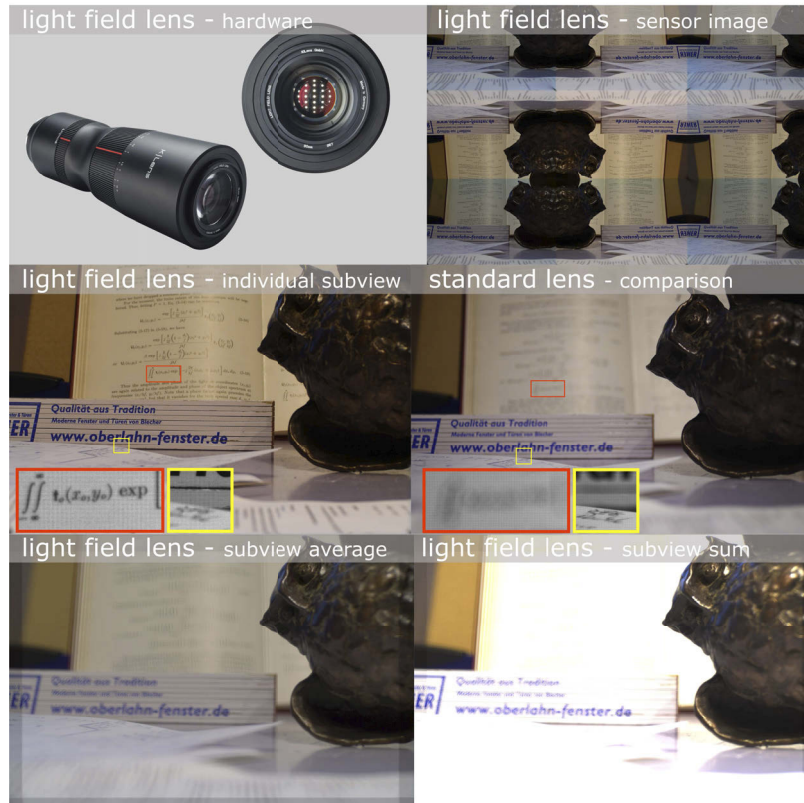
Fig. 4. Kaleidoscopic light field lens “KLens One” with view of the sub-apertures (top row, left), acquired sensor image of the light field system (top row, right), cropped center sub-view of the light field imaging system, equivalent focal length = 78mm, ISO setting= 200, exposure time= 1/10s, insets show raw image content (middle row, left), comparison standard system (St) photograph using a Nikon AF Nikkor 28 – 80mm f/3.3-5.6 G, set to focal length = 75mm focal length, aperture setting = f/6.3 , ISO setting= 200, exposure time= 1/10s, insets show raw image content, note the 3× higher resolution but the much shallower DoF (middle row, right), an averaging of the light field views gives an approximate impression of the digitally decreased DoF available to focus synthesis methods [4], the blur region is slightly larger than in the standard system (St) due to uncompensated sub-view distortions (lower row, left), summation of the light field views demonstrates improved exposure and SNR, e.g. on the body of the owl statue (lower row, right). Raw images used to generate this figure can be found in Dataset 1 [25].
