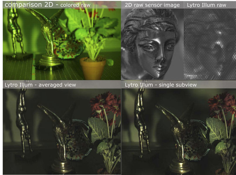
Fig. 6. Comparison standard 2D imaging (Nikon D850, AF Nikkor 85 mm f/1.8; F/\# = 2.2 , exposure time=1/80 s, ISO=100) and Lytro Illum (exposure time=1/100 s, ISO=100, f_{\text{eq}} \approx 80 mm). The output is as “unprocessed” as possible. The colored raw image uses the Bayer pattern brightness assigned to the respective color channel. Raw images are shown as captured. The processed Lytro Illum images have been directly generated from the raw data stored in the .lfp camera file. Only demosaicing and resampling has been applied to the 10-bit output. Note the similar exposure. The DoF is different due to incomparable sensor and pixel sizes. Raw images used to generate this figure can be found in Dataset 1 [25].
