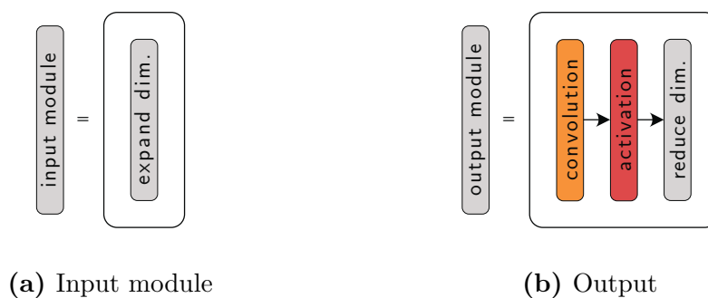
Figure 8.5: Architecture of the necessary embedding modules. These modules are necessary to ensure a smooth IO.
