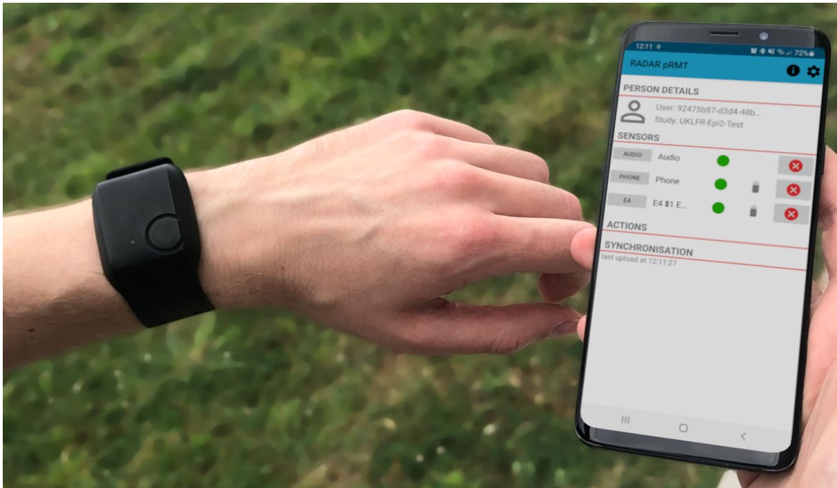
Figure 5.4: One of the Empatica E4 wrist-worn wearable devices used in this study ( left ), and the Android phone application that connects to the wearable via Bluetooth and records the data stream ( right ).
