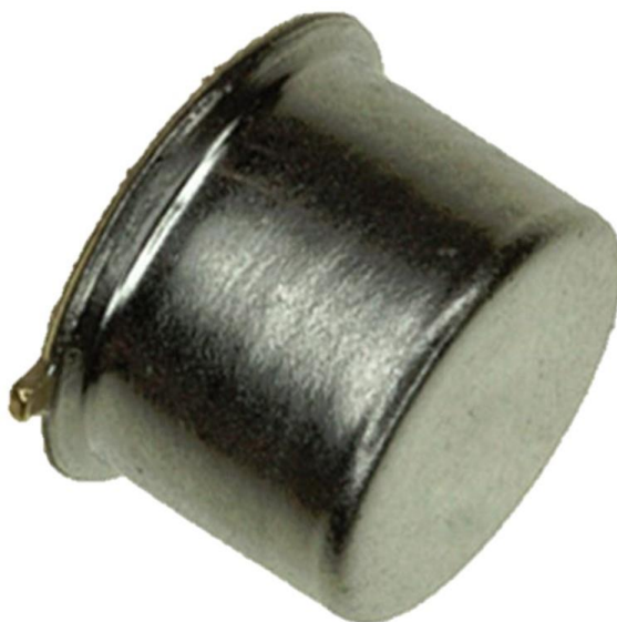
Figure 3.1: Sampling device and sample carrier for blotting technique [79].
