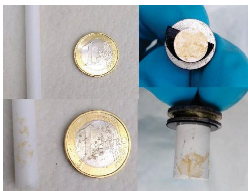
Figure S11: ZrNT film transferred to different surfaces. L: plastic rod and €-coin without {top} and with {bottom} transferred ZrNT layer. R: flat {top} and curved {bottom} surface of ZrO_2 -rod.
