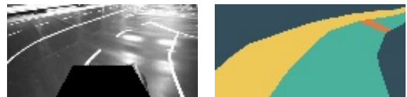
Figure 6: Example of a real world image (left) with its manually annotated label (right) from the test dataset.
