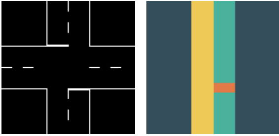
Figure 2: An image with its annotation representing an intersection chunk. The pixels of the image are assigned to a semantic class by their color (class 'left lane': yellow, class 'right lane': green, class 'obstacle': red, class 'intersection': orange).
