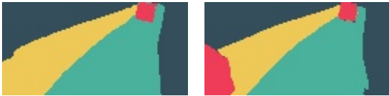
Figure 9: Two different predictions from the image in figure 8: The image on the left is a segmented output of a network trained only on real world data. On the right is the output of a network trained with synthetic and real data. This example demonstrated how synthetic data improve the classification of the under-represented class 'obstacle'.
