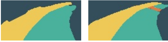
Figure 7: Two different predictions from the image in figure 6: The image on the left is a segmented output of a network trained only on real world data. On the right is the output of a network trained with synthetic and real data. This example demonstrated how synthetic data improve the classification of the under-represented class 'intersection'.
