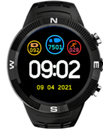
Figure 2.3 Bangle.js 1 Smartwatch with our Activate firmware installed. The display indicates the battery charging level, the number of steps taken during the day, and the number of active minutes [104].
