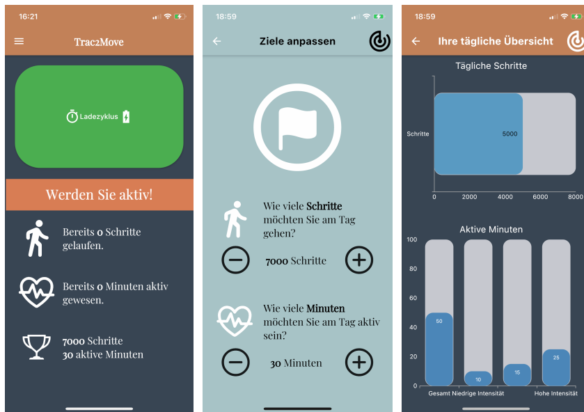
Figure 3.4 The smartphone's user interface: (1) Home Screen, (2) Setting daily activity goals, e.g. Daily Steps (Tägliche Schritte) and daily Active Minutes (Aktive Minuten), (3) Graphical overview of daily activities: Daily Steps (Tägliche Schritte), Active Minutes (Aktive Minuten), divided into three intensities - low, moderate and vigorous (niedrige, mittlere, hohe Intensität).
