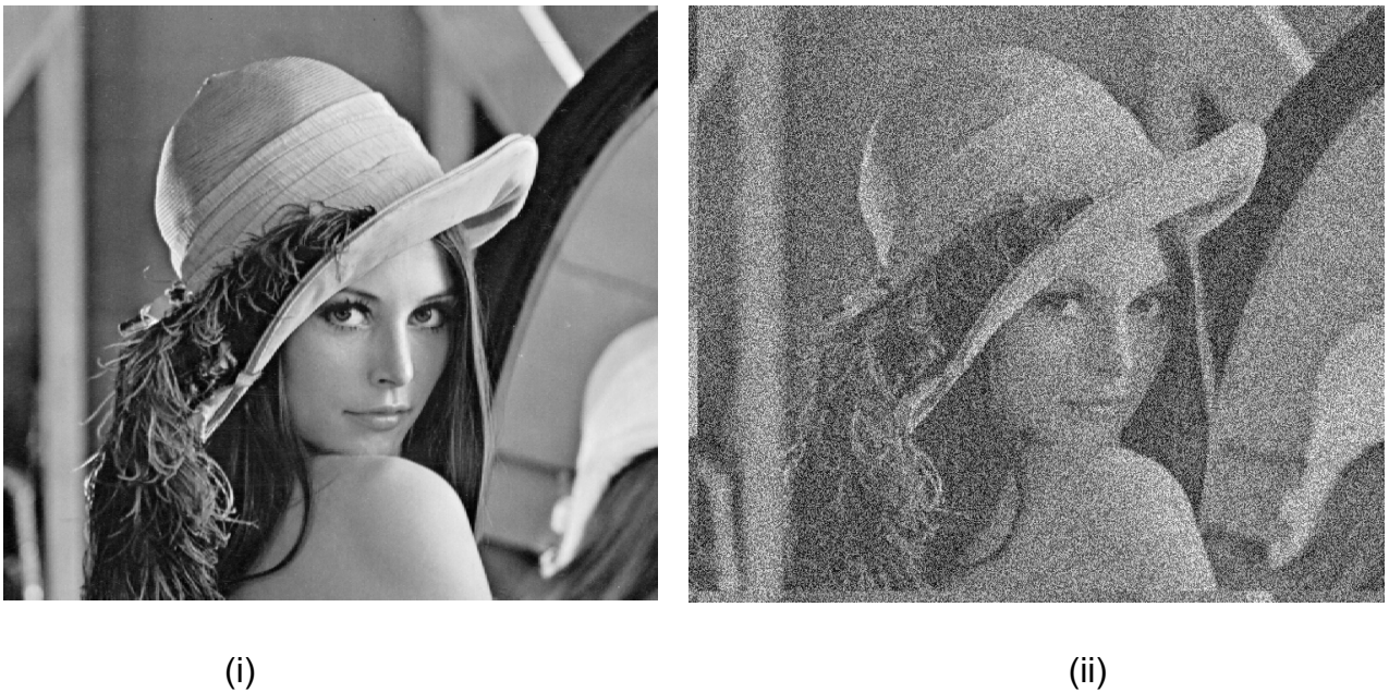
Figure 5.1 Reference image (i) and after adding Gaussian noise of SNR 10dB to image (ii)
