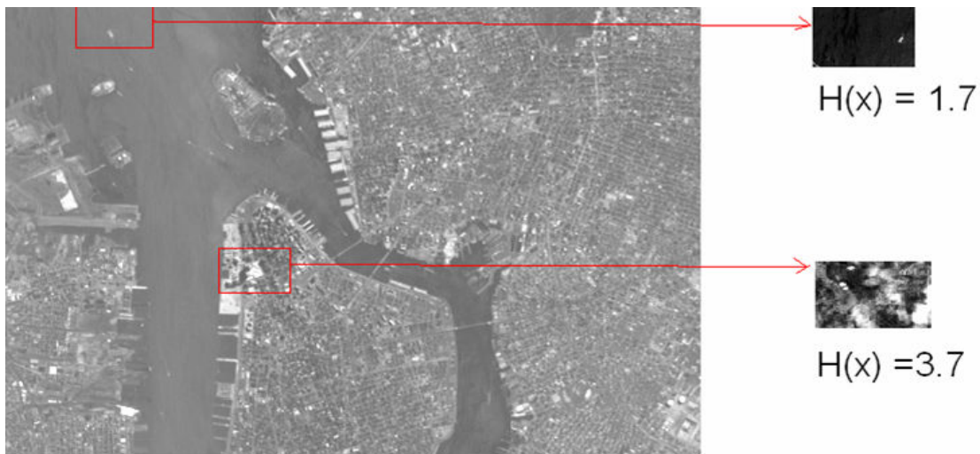
Figure 2.2 Image showing subimage with highest and lowest entropy respectively. The image was divided into 64 parts. The entropies of each of the 64 subimages were calculated. The subimages with the highest and the lowest entropies are selected
