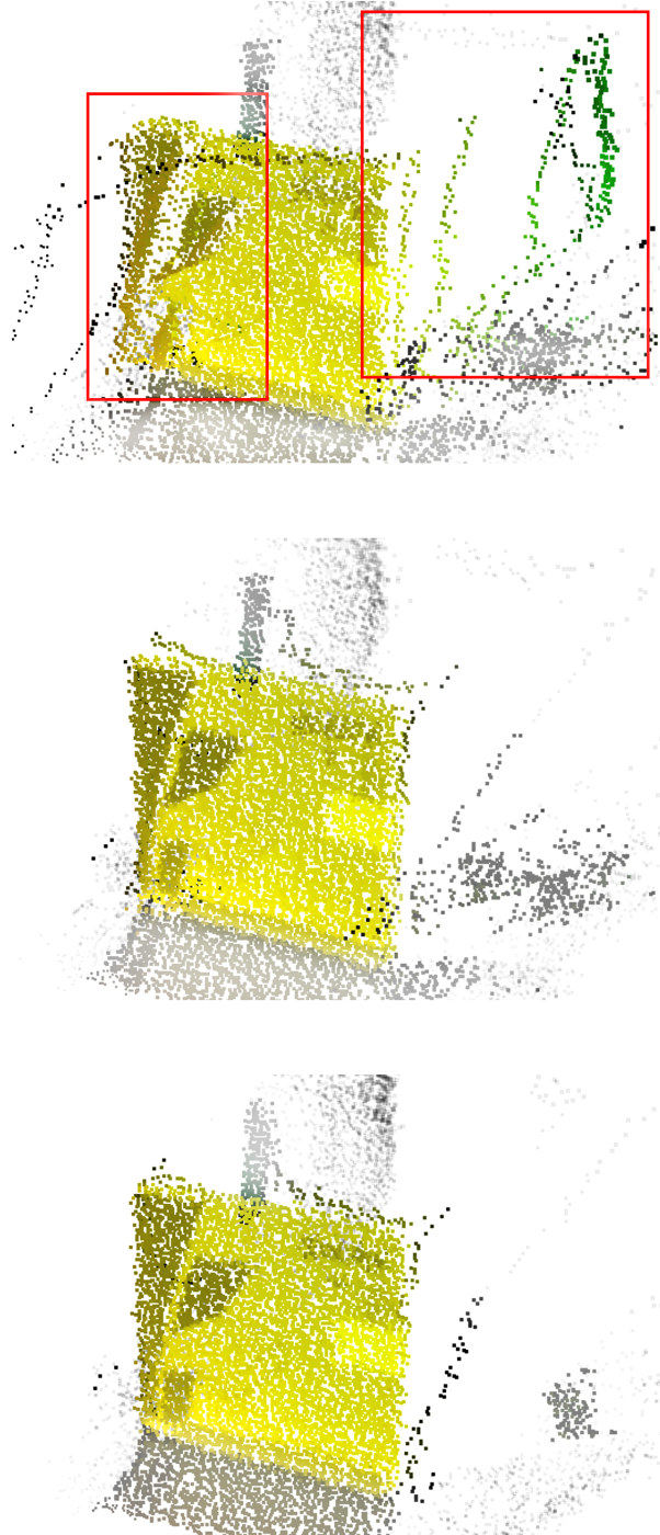
Figure 2.15: Scene 1 before (top) and after motion compensation (middle) as well as the static reference scene (bottom). Note the motion artifacts due to texture changes of the box surface.
