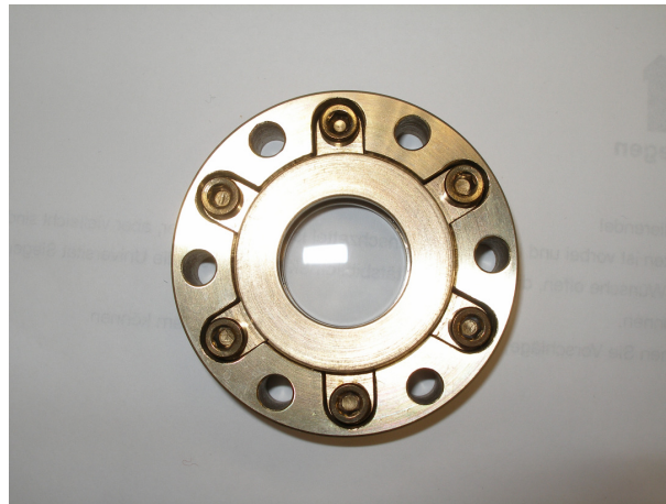
Figure E.2: Laser viewport on the CF40 flange.
