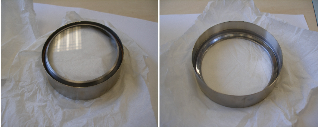
Figure E.1: Viewport sub-assembly. This part was separately anti-reflection coated for the 369 nm UV light and later mounted onto the CF100 flange.
