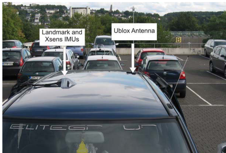
Fig. 7.9 Mounted IMUs and GPS antenna on car roof
