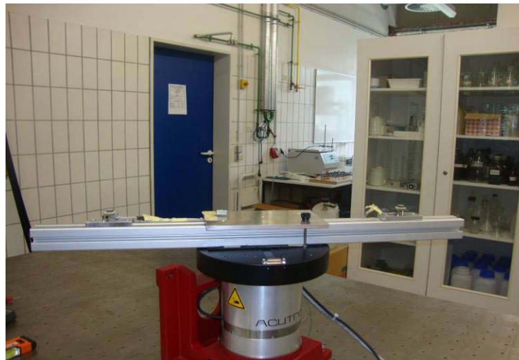
Fig. 4.3 Reduced configuration of rotating accelerometers using turntable
