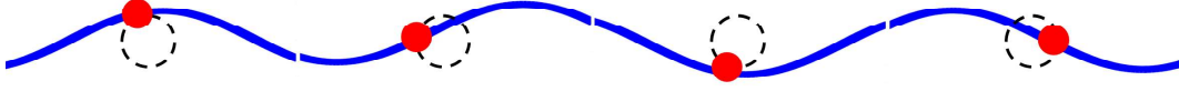
Figure 3.3: Orbital velocity for deep water assumption. Particle moves along a constant circle in dependency of the position on the gravity wave. The wave moves in the right direction.
